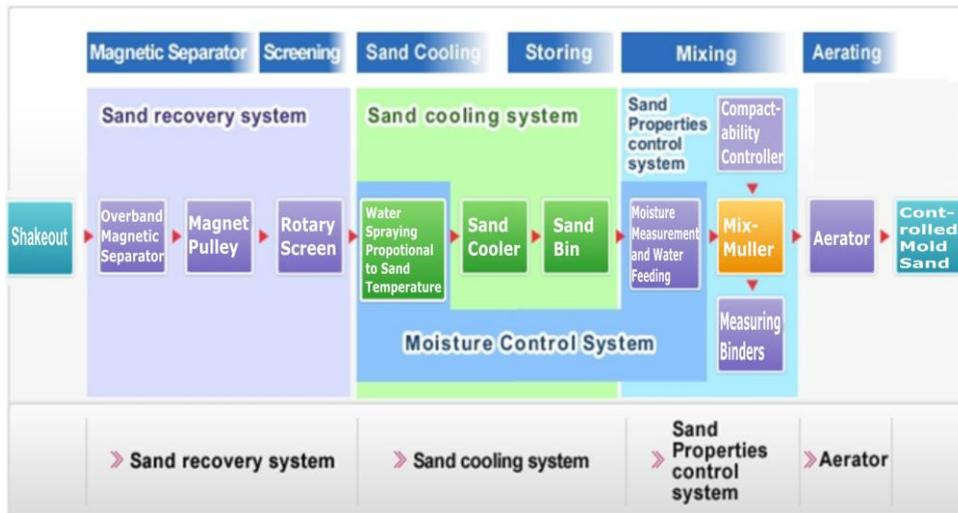
Fig.1 Flowchart of the Standard Green Sand Treatment System
