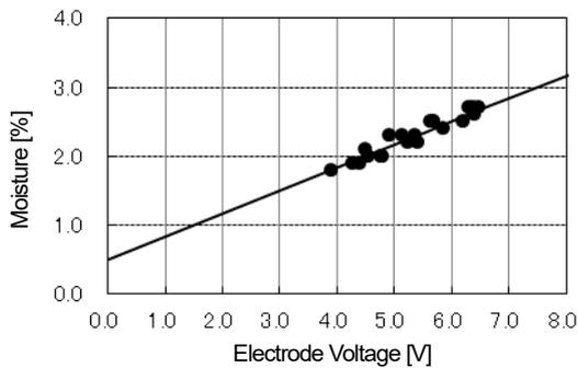
Fig. 8 Calibration curve for Conventional System
