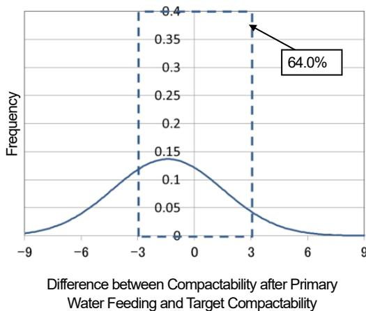
Fig. 11 Compactability Measurement Result in Conventional System
