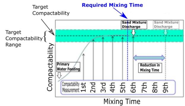
Fig. 7 Compactability Transition in Developed System
