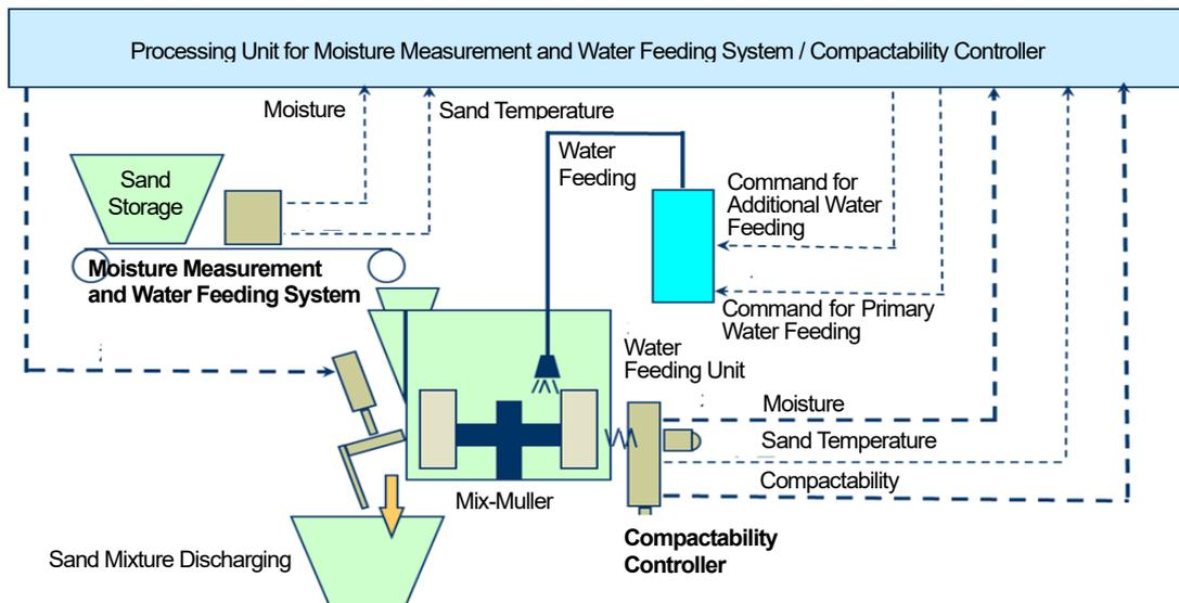
Fig. 5 Sand Mixture Control System
