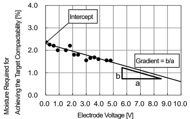
Fig. 9 Function for Determining Required Water Amount on Primary Water Feeding in the Developed System
