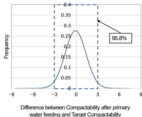
Fig. 12 Compactability Measurement Result in Developed System
