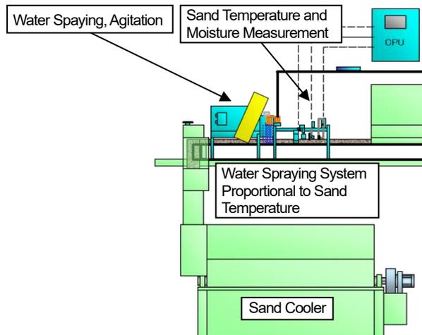
Fig. 2 Configuration of Conventional Sand Cooler
