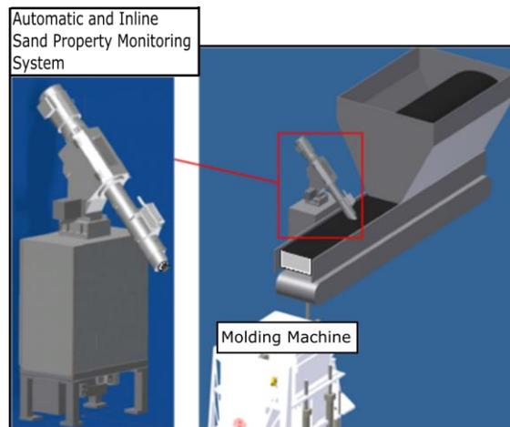
Fig.13 Outside View of Automatic and Inline Sand Property Monitoring system and Situation to be Built Inline
