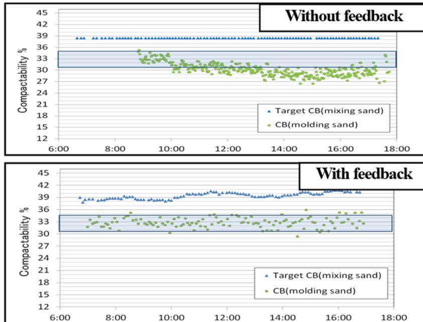
Fig.14 Compactability on Molding Machine With/Without Feedback Control
